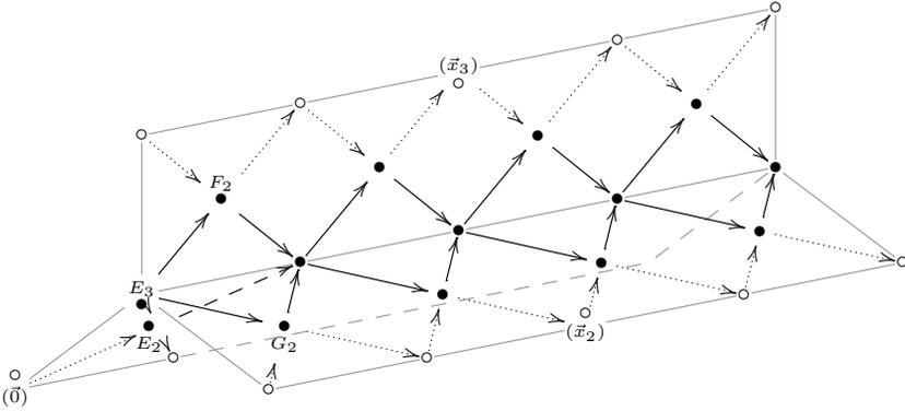
For each  $\tau$ -orbit of line bundles, we select one member, in bracket notation the line bundles  $\mathcal{O}$ ,  $\mathcal{O}(\vec{x}_2)$  and  $\mathcal{O}(\vec{x}_3)$ . Also, as indicated in the figure, for each of the four remaining  $\tau$ -orbits, we select one member, resulting in three rank-two bundles  $E_2$ ,  $F_2$  and  $G_2$  and one bundle  $E_3$  of rank three.
